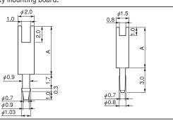
KB type (for fitting hole diameter of  $\phi$  0.8)
