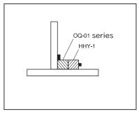
By using OQ-01 series, the SMT boards can be mounted at right angle.
