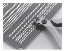
Cut it by using a nipper when it becomes unnecessary
