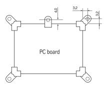
•Please insert EP series underneath to raise 1.5 mm or over from the chassis (base).
