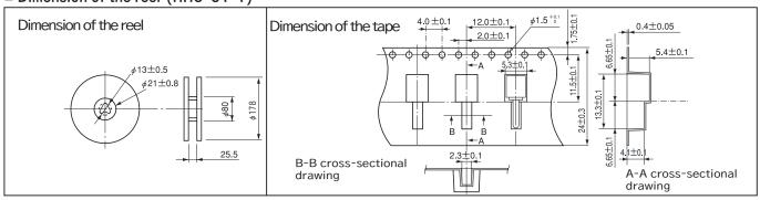
X The dimension of the reel for HH-51-T is the same as that for HH-5.
