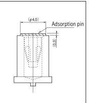
Adsorption pin is attached for the tape-and-reel. After soldering, please dispose it.
